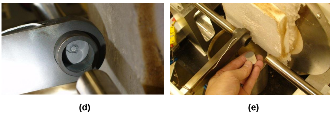
Figure 13. Different stages in the installation of an iridium specimen.
