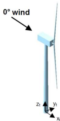
Figure 11. Tower Base Coordinate System (Jonkman and Buhl 2005).
