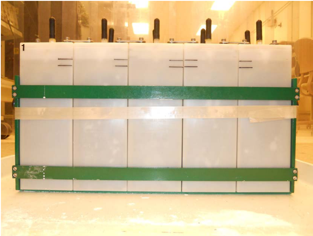
Figure 1. Encell Phase I Battery pack as received for testing.
