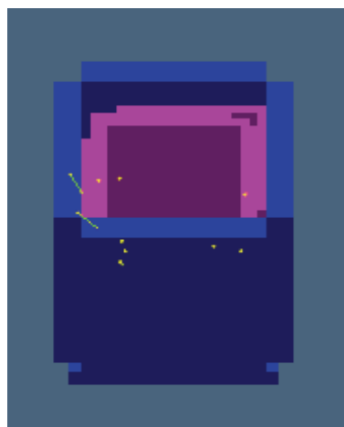
Figure 7 IO8 contains plutonium (purple) shielded by depleted uranium (light blue).
