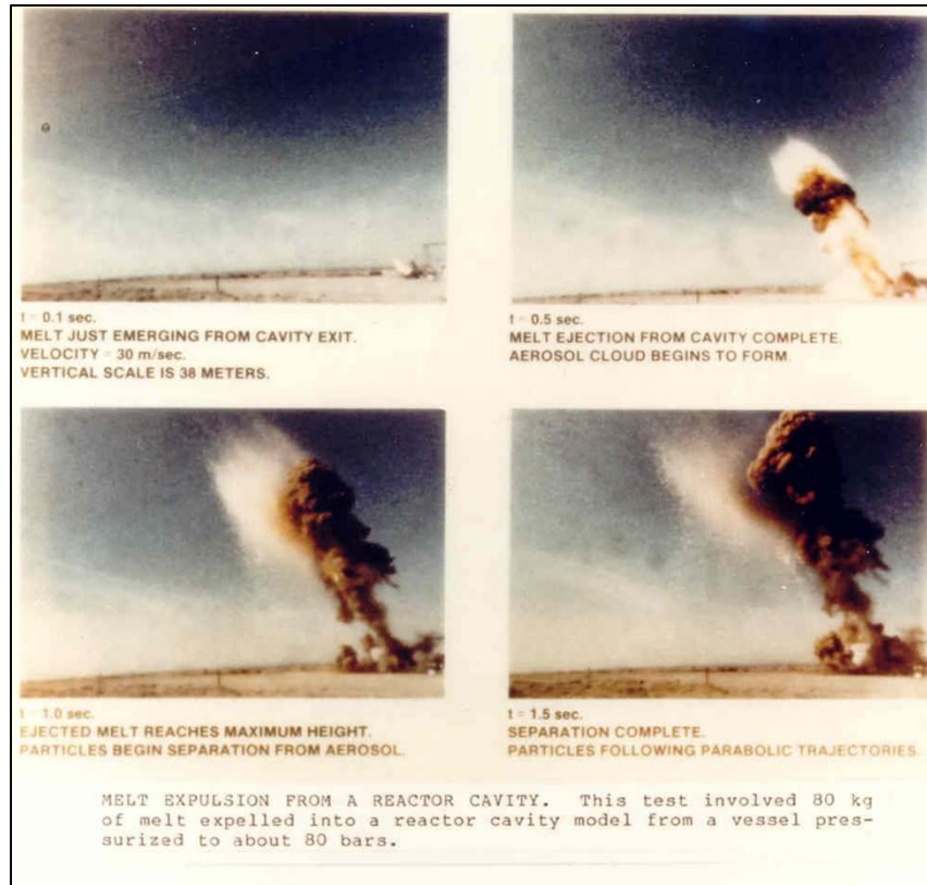
Figure 4: Sandia Experiment Characterizing Containment of Thermal Loads
