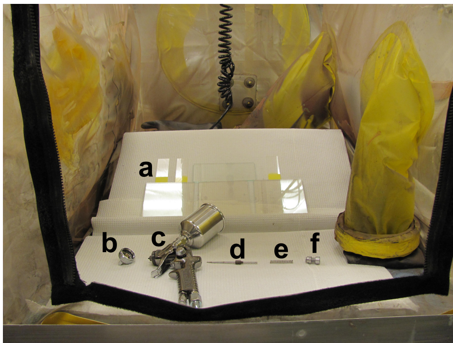
Figure 6. Image of spray equipment inside the HEPA-filtered tent. Identified parts are described in detail in Table 3
