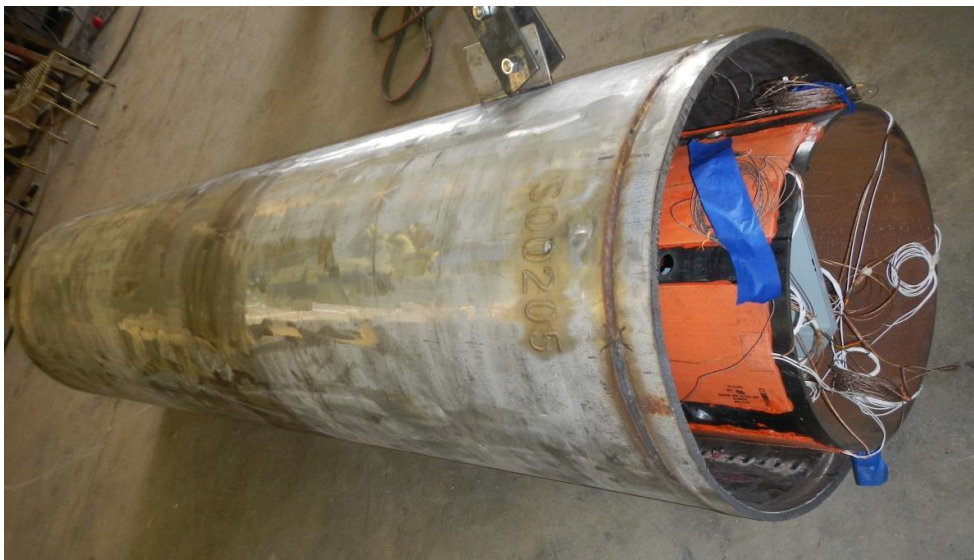
Figure 18. Heating harness inserted into canister.
