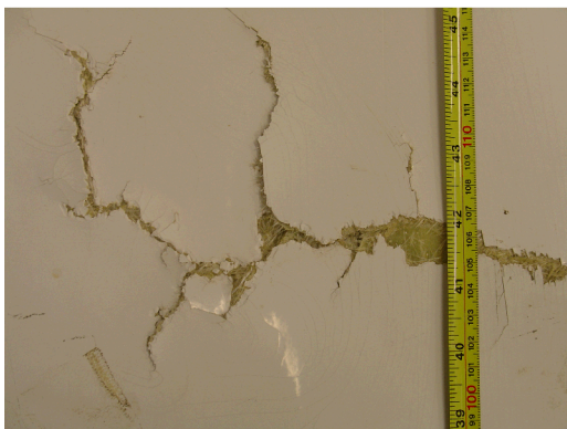
Figure 24: Crack near blade centerline on TX-100 blade.
