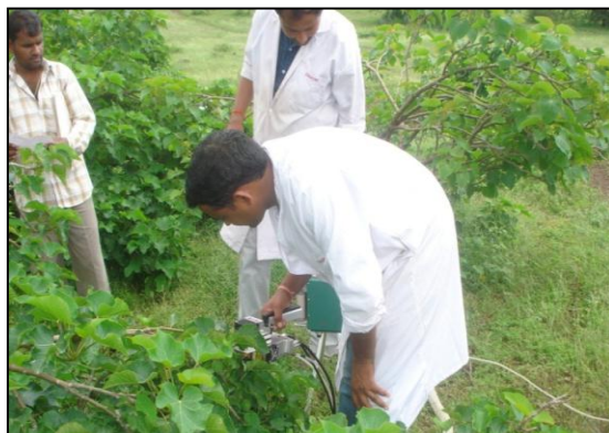
Figure 47. Gas exchange measurements like photosynthesis, transpiration, stomatal conductance being taken with the help of Infra-red gas analyser system (LI-COR, USA).
