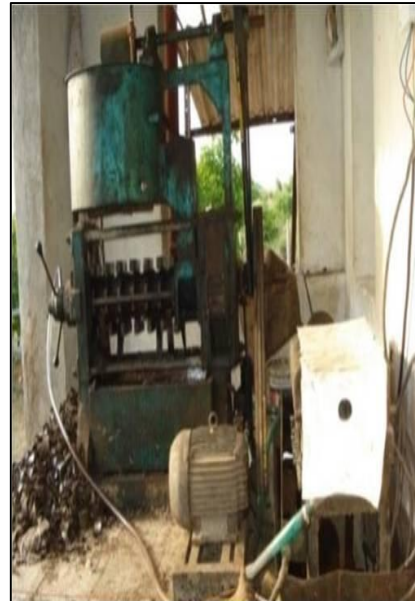
Figure A10. Expulsion of oil from Jatropha seeds and generation of oil cake in a unit
