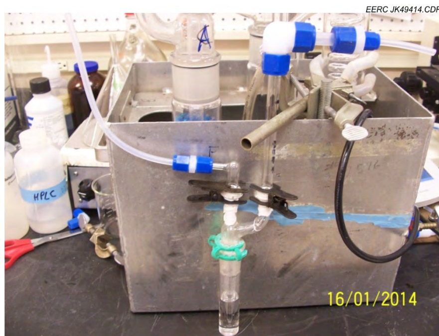
Figure 4-5. Photograph showing the midjet impinger for Method 3509 sampling. During sampling, the impinger is located inside the metal box.
