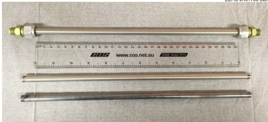
Figure 6-11. As-received tube (bottom), Pd-coated membrane (middle), and a membrane sealed with compression fittings (top).
