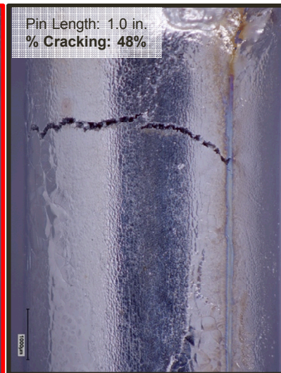
Terminal eutectic phase decorates fracture surface of Ni-51Ti CPTT
