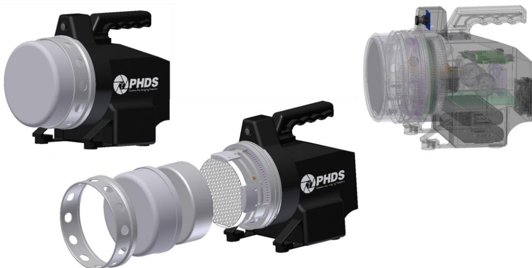
Figure 11: The full GeGI-DNN design was completed during Phase I. The GeGI-DNN will be compact and lightweight, with dimensions of 7" diameter and 11.5" long and a weight of 18 lbs.
