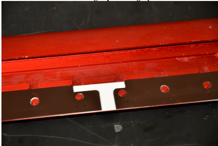
Figure 9. Close-up of Alstom foil interior with blocking shims
