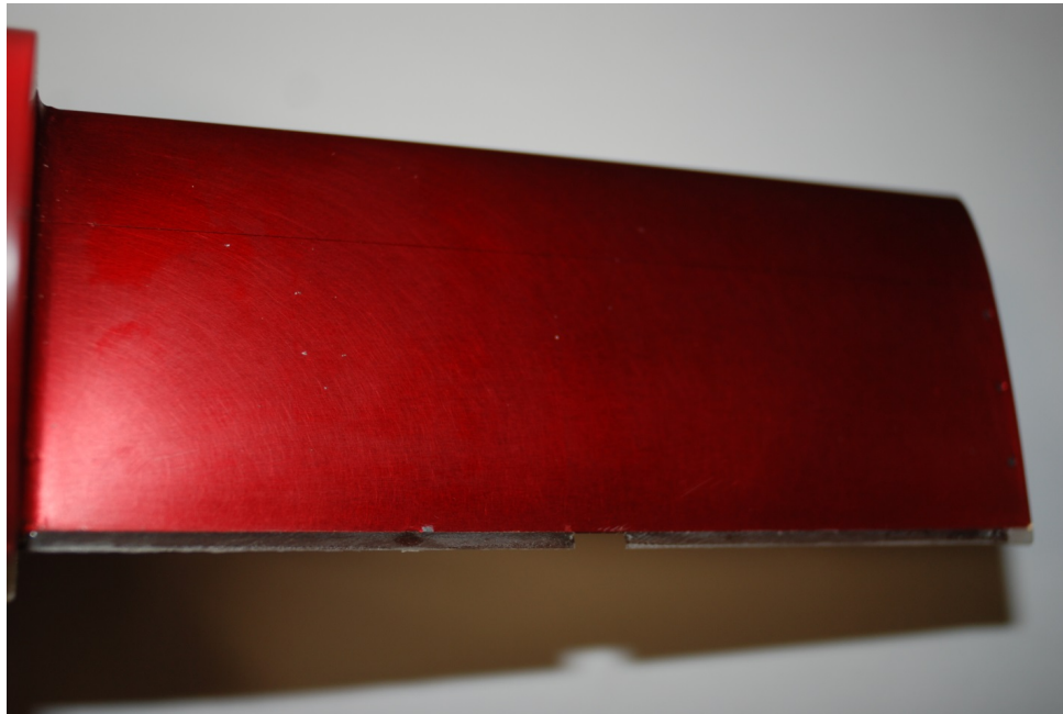
Figure 11. Alstom foil with extended blocking shims and epoxy filling of trailing edge
