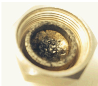
Figure 7: Swagelok cap with fouling product from the turbo-alternator-compressor (TAC) unit in the RCBC.
