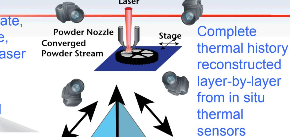
Complete thermal history reconstructed layer-by-layer from in situ thermal sensors
