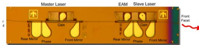
On-Chip Injection Locking Enhanced Modulation > 50 GHz, C-Band
