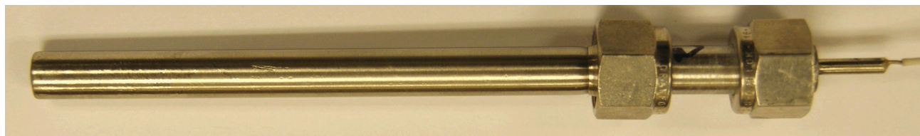
Figure 2. (a) Schematic drawing of a ruggedized high temperature and pressure stable iodide ion selective electrode (I-ISE). (b) Photograph of the I-ISE.
