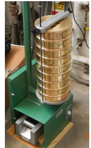
Flow that was drained was diverted through sieves for collection and weighing
