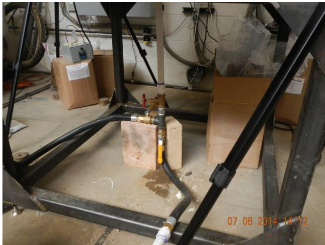
Valves to divert flow from filling to draining
