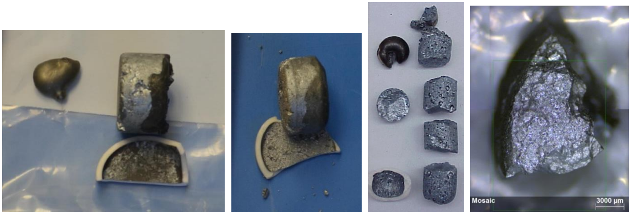
Figure 2. ASM (left), Birchenall (second), FactSage (third) compositions of CuMgSi, including bottom portion of crucible. Broken piece of ASM sample (right) shows the dark discoloration was limited to the surface
