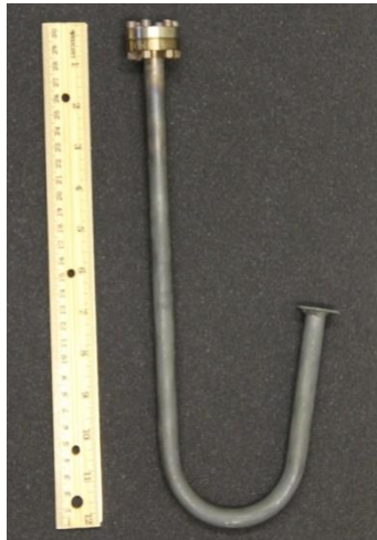
Figure 10. In625 configuration for materials screening tests. PCM is located in curved portion of the tube.
