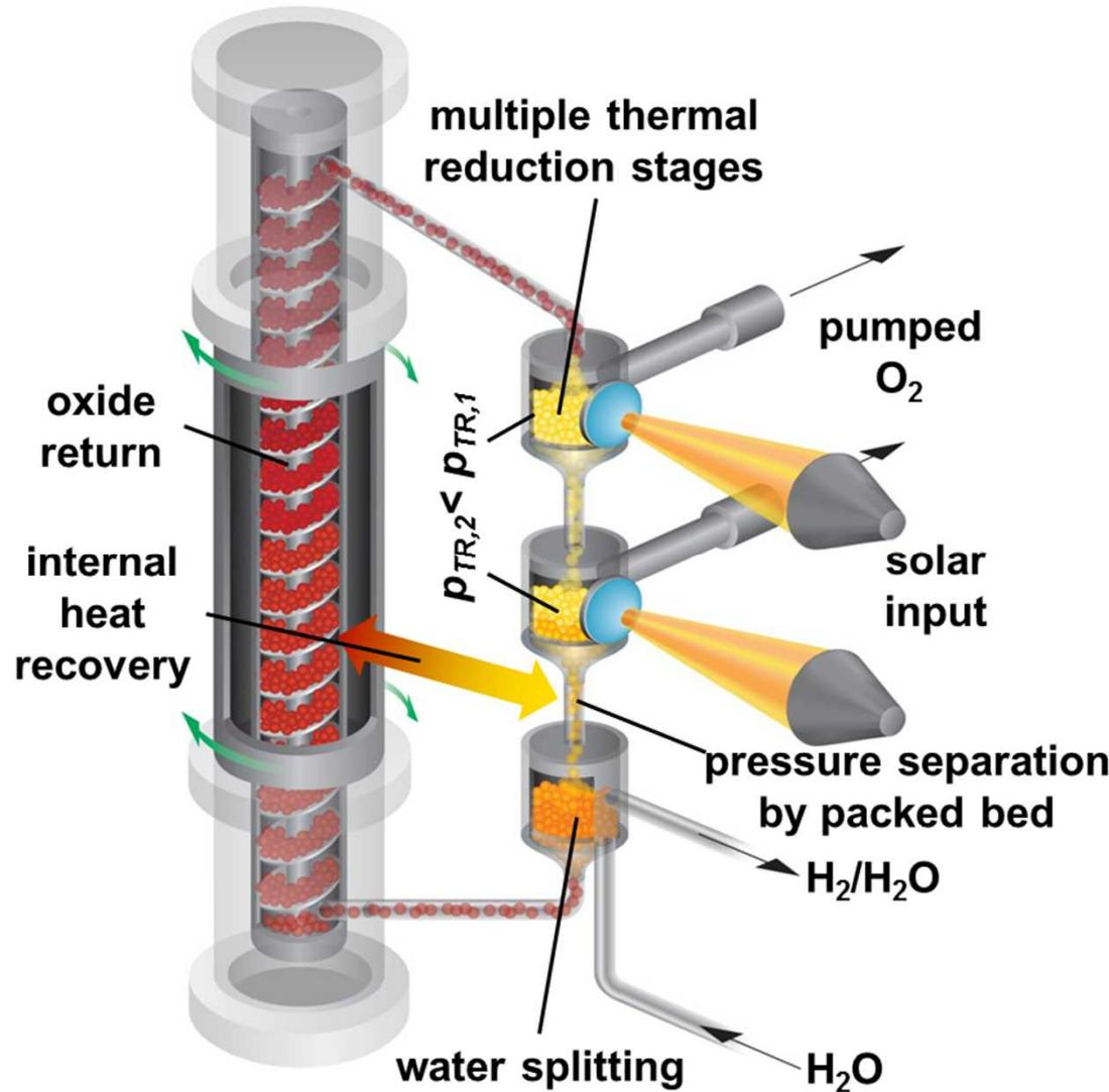
Incrementally pumping  $O_2$  reduces the overall flow volume and velocity
