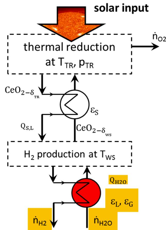
Low  $\Delta T$  or high reduction pressure leads to a high steam/H<sub>2</sub> ratio
