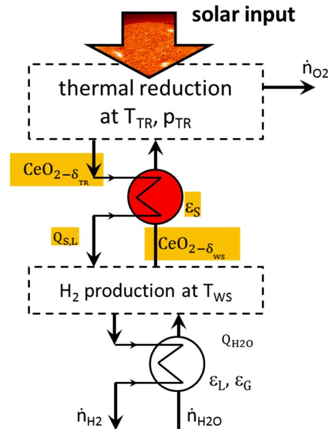
A low reversible oxygen capacity leads to a very high oxide/ $\text{H}_2$  ratio and excessive oxide mass flow and heat recovery requirements
