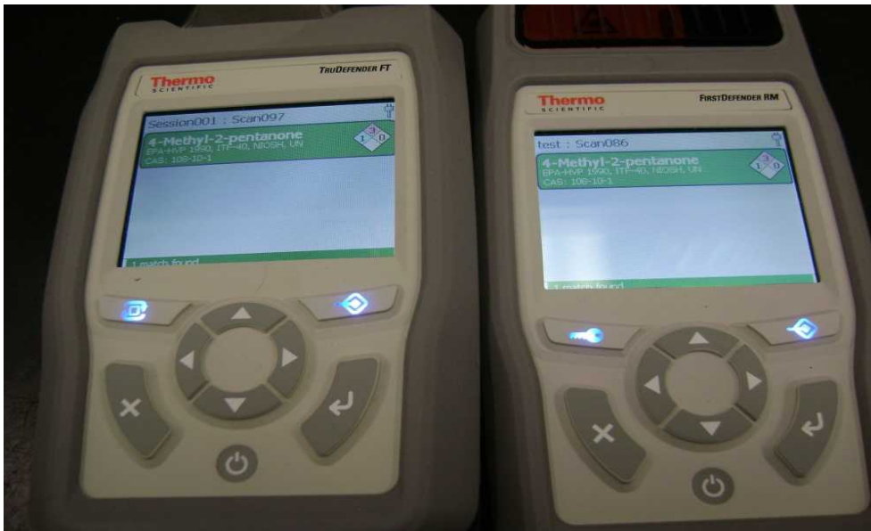
Figure 1: A comparison of the hexone sample results as seen on the TruDefender FT and the FirstDefender RM
