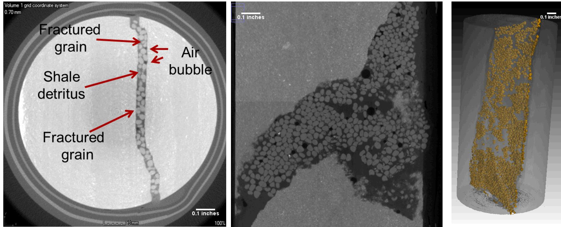
X-ray  $\mu$ CT data allows us to investigate the effects of the application of pressure, temperature, and pore fluids on cracks and proppant particles. Grain fracturing, embedment and shale fracturing was observed.
