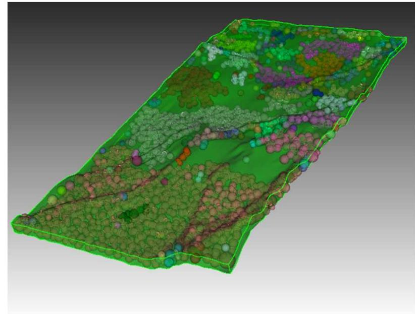
Combine particle size and location information with crack geometry by generating spheres at appropriate locations → possible to generate high-quality mesh that accounts for particles: (Still in progress)
