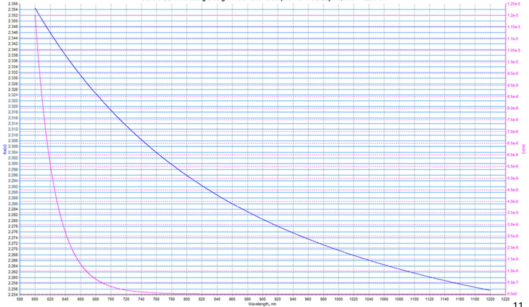
Sandia BBHR Coating Design: Index and Absorption of TiO 2 Layers, 600 - 1200 nm
