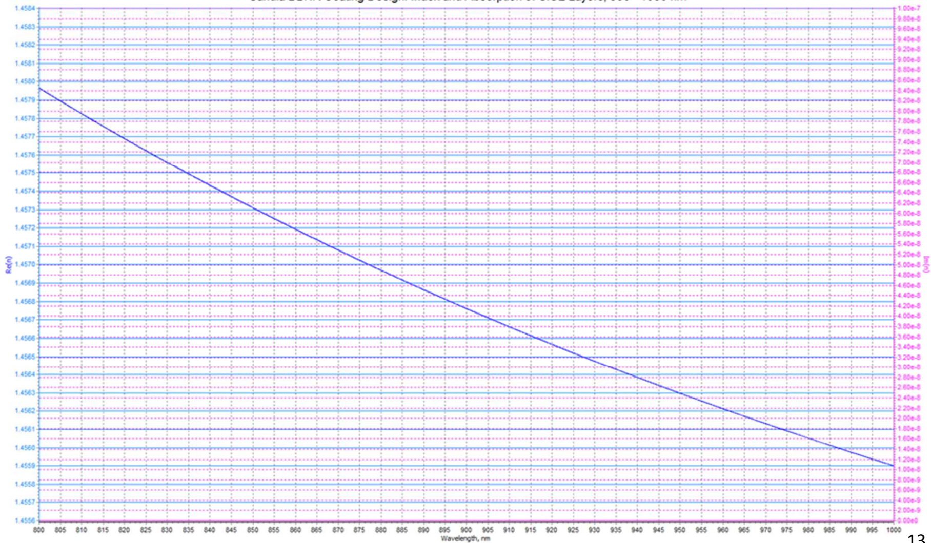
Sandia BBHR Coating Design: Index and Absorption of SiO 2 Layers, 800 - 1000 nm
