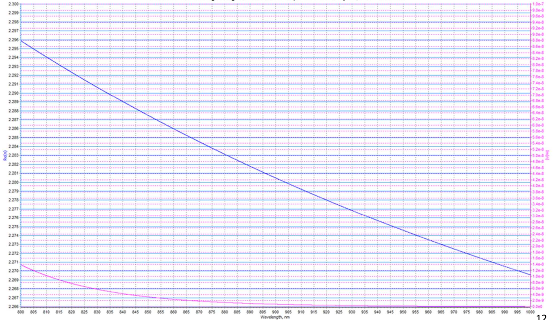
Sandia BBHR Coating Design: Index and Absorption of TiO 2 Layers, 800 - 1000 nm
