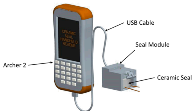
Figure 7: Handheld reader concept. Reader connects to Ceramic Seal via “tag-connect” on seal cap, providing in-situ information on seal status such as SOH and events. Image courtesy SRNL.
