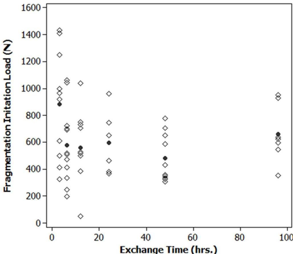
1. The average load to cause cracking during loading is approximately identical
