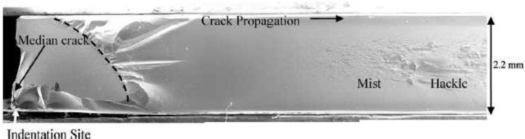
Montage of images showing the fracture surface for a 24 hr., 450°C sample loaded monotonically to fracture. Bottom left is the fracture origin. The crack pops-in, propagates through the thickness, and then sweeps through the sample, from left to right.
