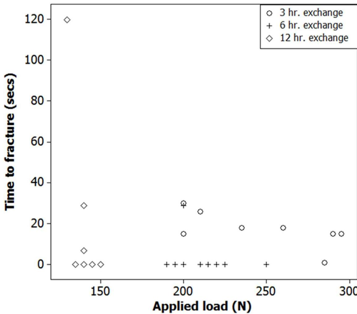
2. Load required to cause cracking during/after unload is highest for the smallest exchange times
