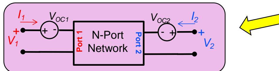
Excluding the port loads, **linear** time or frequency domain EM simulators are used to determine the **open-circuit voltage** and **impedance parameters** at the ports.
