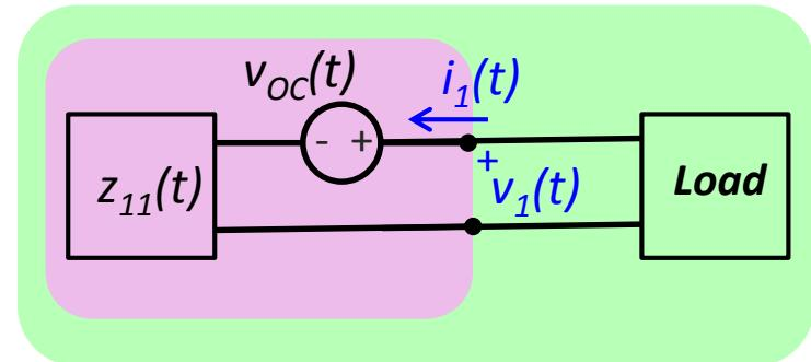
For distributed coupling problems the self-impedances ( $z_{mm}$ ) are impulsive near  $t=0$ .
