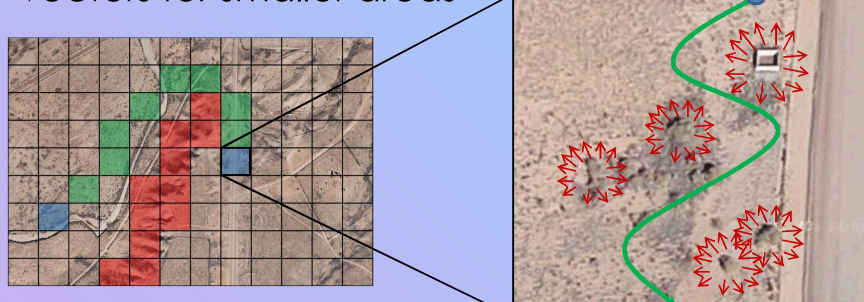
The D\* search algorithm will find the optimal path, with respect to terrain difficulty, that our robot should travel.
