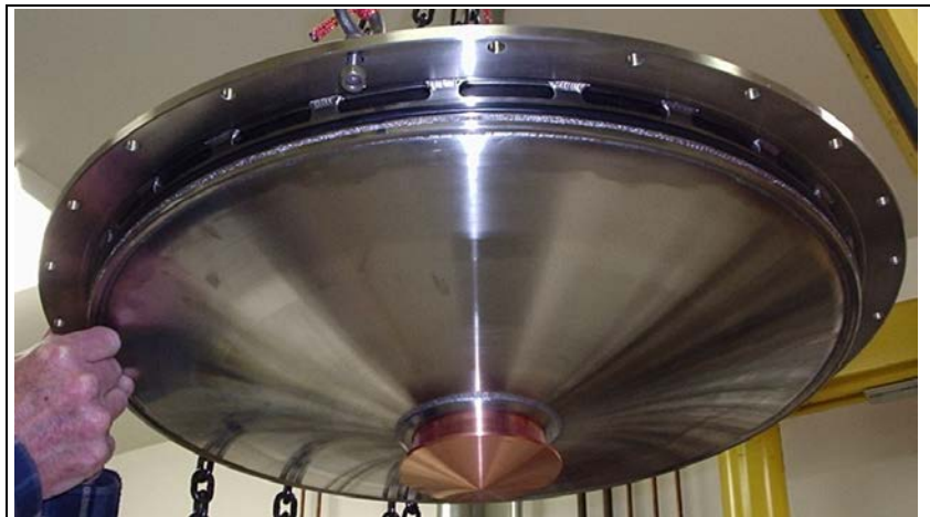
Figure 18. Stainless steel end plate for DOE-ITER load, including copper sieve vacuum port
