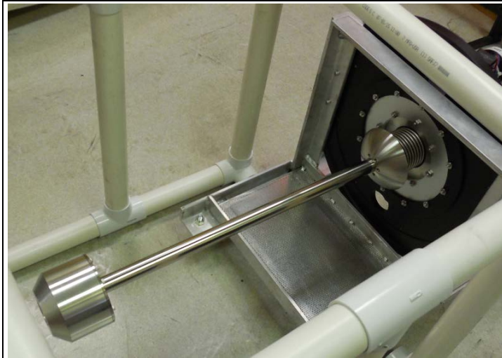
Figure 7. Test revolving reflector assembly in test structure
