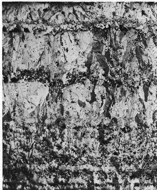
Figure 26. GEM ZIRCONIUM CARBIDE DEPOSITED IN RUN 5 AT 52 INCHES AND AT 1,400°C. (Bright Field Illumination; 75X)
