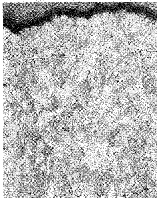
MS 71-1009-1 Figure 25. GEM ZIRCONIUM CARBIDE DEPOSITED IN RUN 5 AT 37 INCHES AND AT 1,330°C. (Bright Field Illumination; 100X)
