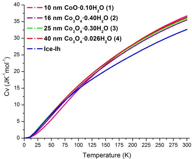
We have also used results from the INS spectra to develop the vibrational density of states (VDOS) from which we are able to calculate the thermodynamic properties of the hydration layers confined to the surface of metal oxide nanoparticles. An example of the calculated heat capacities for Co-oxides is shown to the right.
