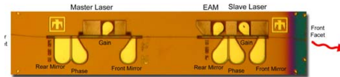
On-Chip Injection Locking Enhanced Modulation > 50 GHz, C-Band
