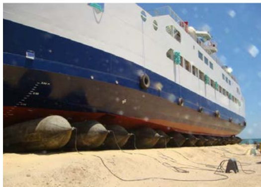
Fig. 11 – Ship launch using rubber airbags [7]
