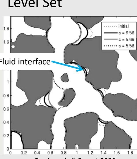
Flow of "frac" fluid in proppant-containing fracture
