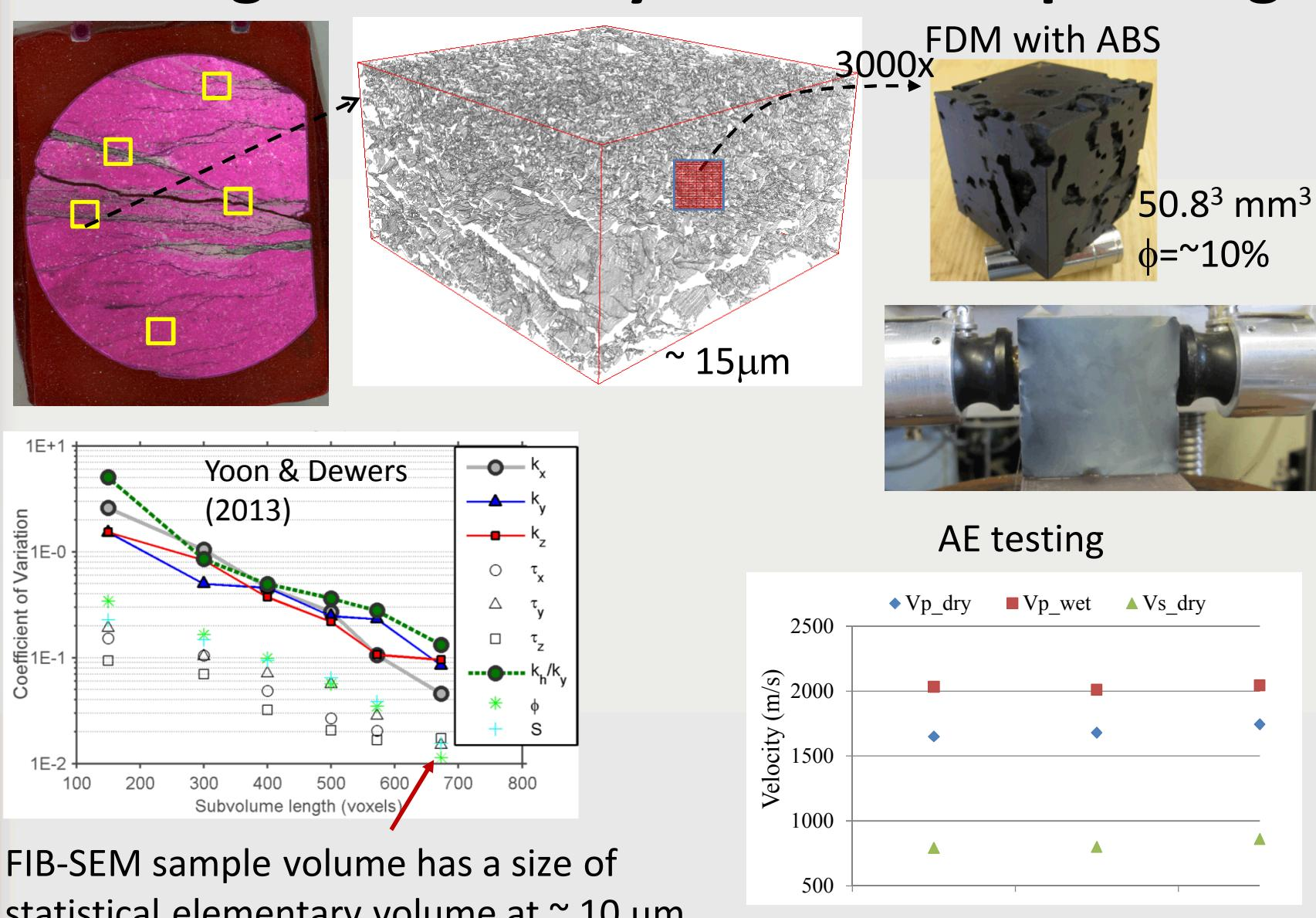
FIB-SEM sample volume has a size of statistical elementary volume at  $\sim 10 \mu\text{m}$
