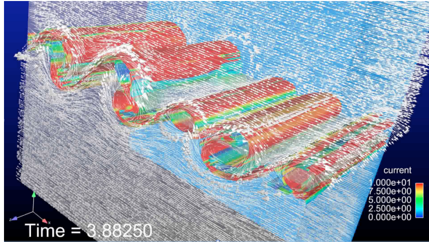
Fig. 8. Hydromagnetic Kelvin-Helmholtz Problem with Re = 10^4 , Re_m = 10^4 , M_A = 3 . Vectors show magnetic field and surface is of constant vorticity colored by the plasma current.
