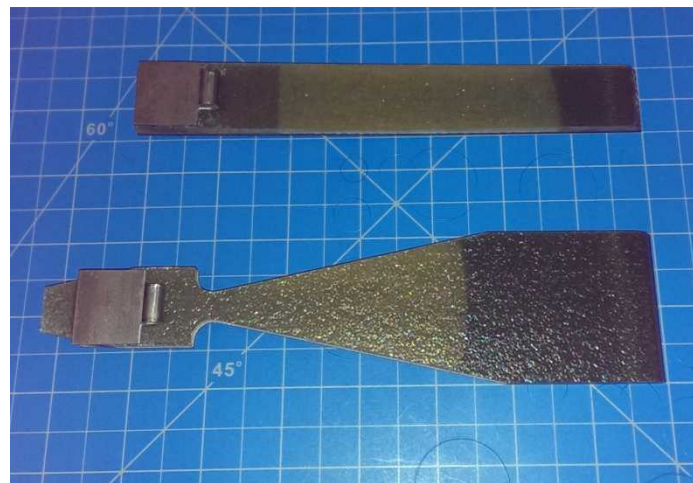
Figure 6. Finished fixed width and width-tapered DCB specimens
