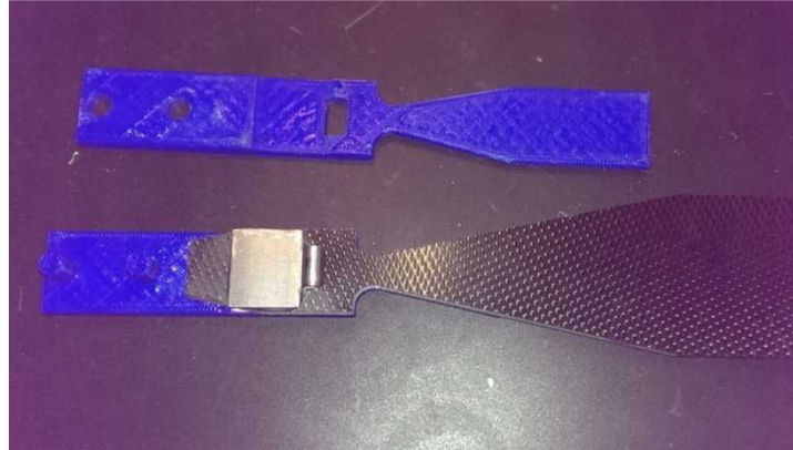
Figure 5. 3D printed hinge bonding alignment fixture
