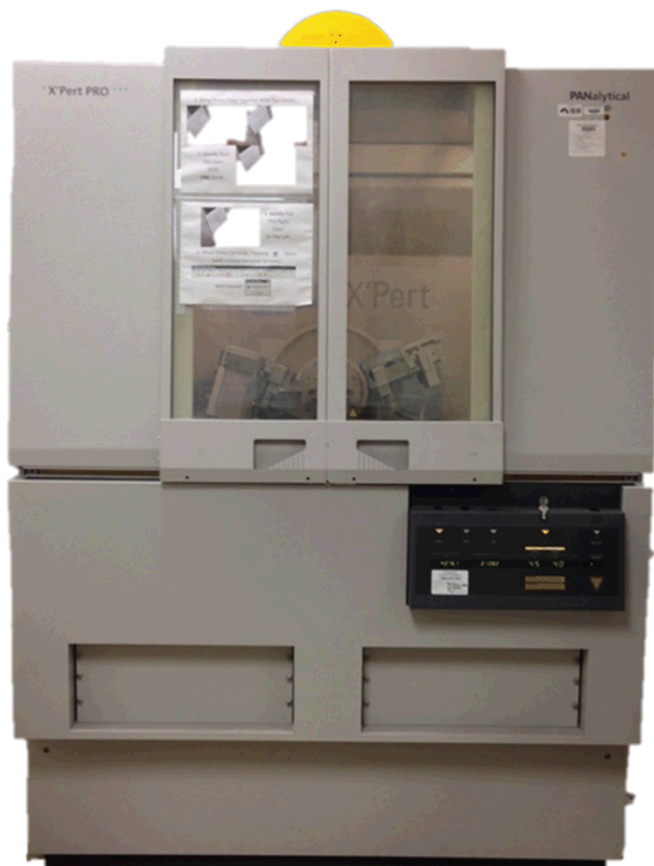
PXRD (Powder X-ray Diffraction): Identifies crystal structure & phase
