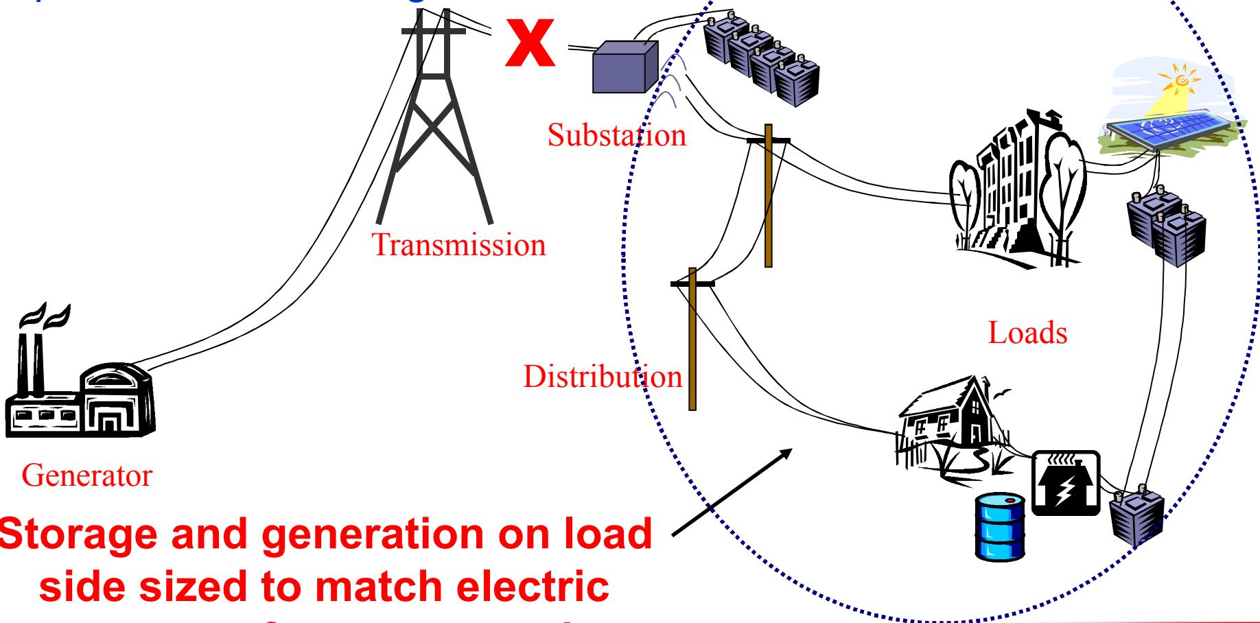
**Storage and generation on load side sized to match electric power performance needs**
