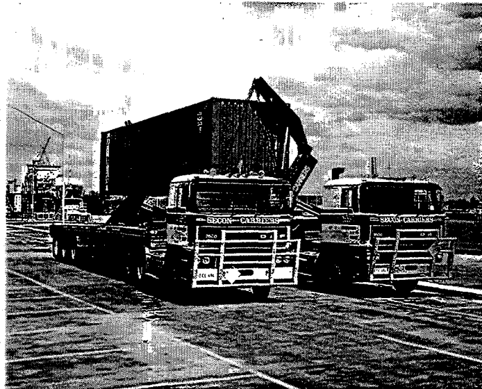
Companion vehicles can drive past the MK6 Sidelifter due to its extended reach
