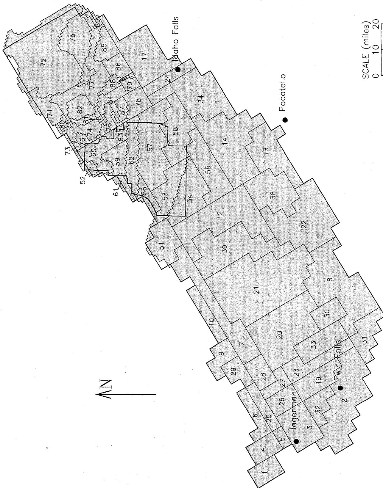
Figure 3-16. Hydraulic conductivity zones defined in the current model.
