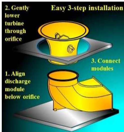
3-Step installation of turbine-generator and discharge modules
