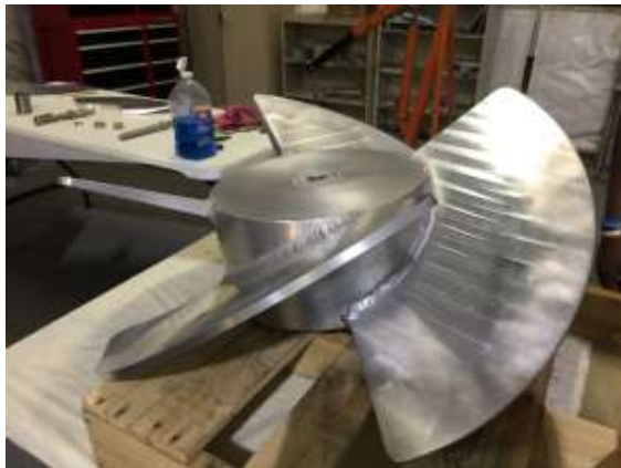
Figure 13a. 30° blade angle, 4-blade Aluminum impeller
