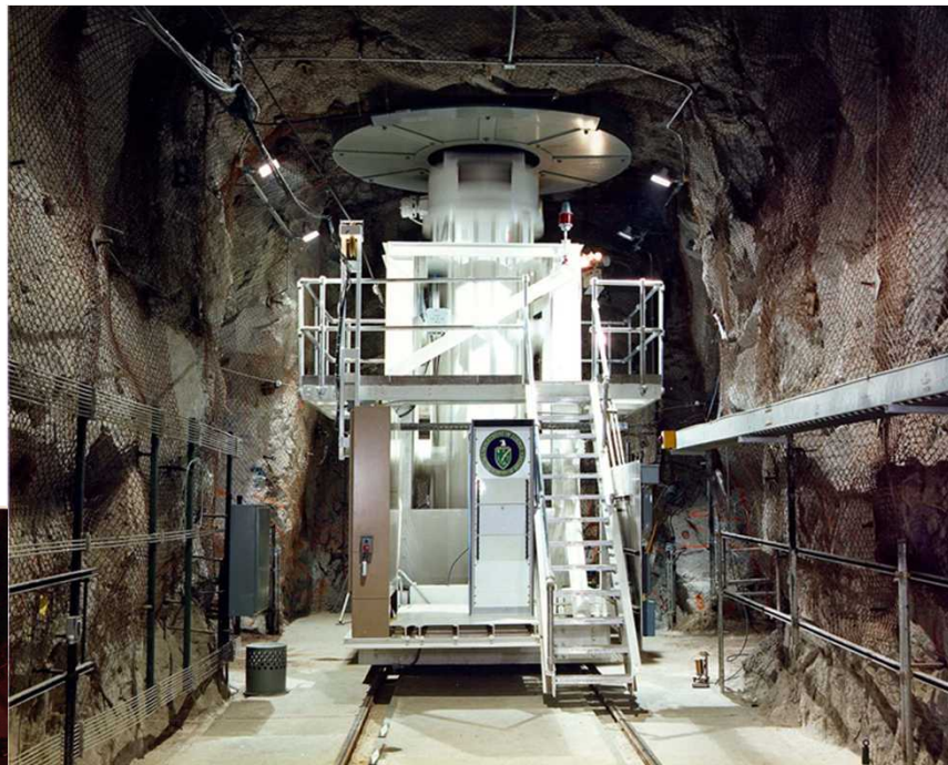
Rail-mounted Underground Transfer Vehicle (in receive position under waste handling borehole)
