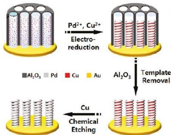
Figure 4. A diagram of the process that Liu et al used to create pure palladium nanosprings 16 .
