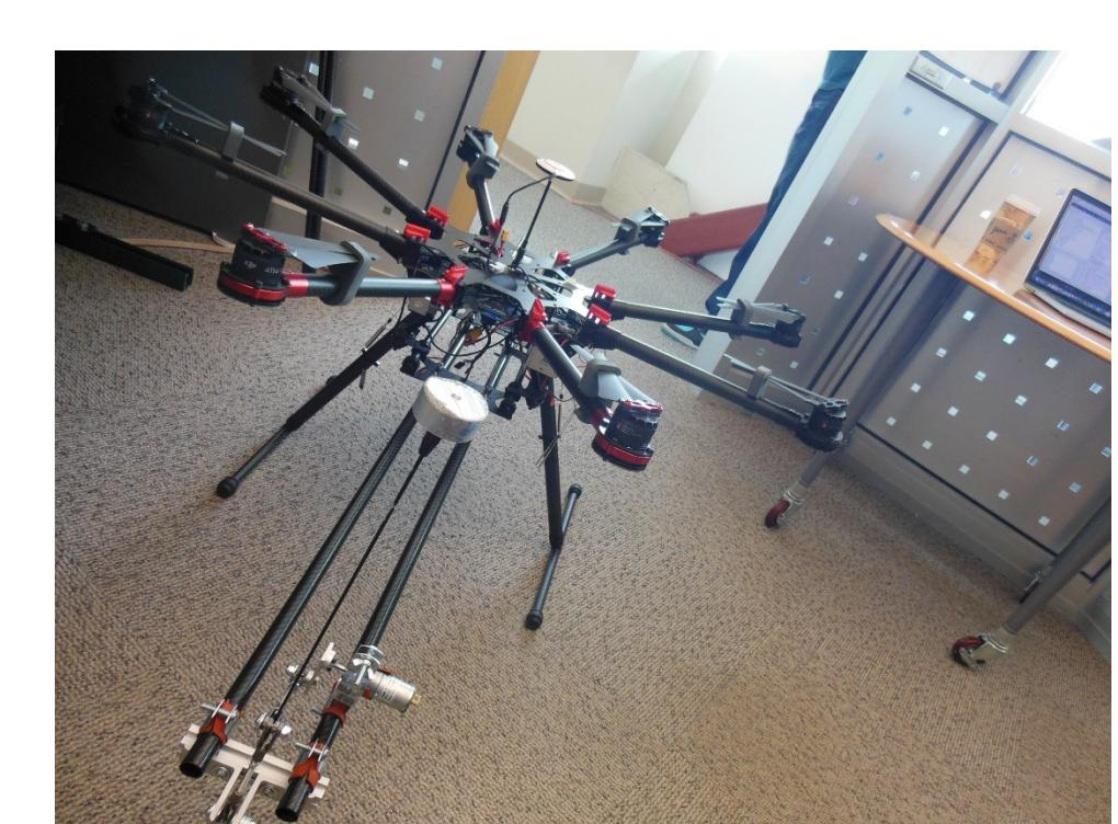
Hammer is rotated to avoid collision with the drone propellers.
