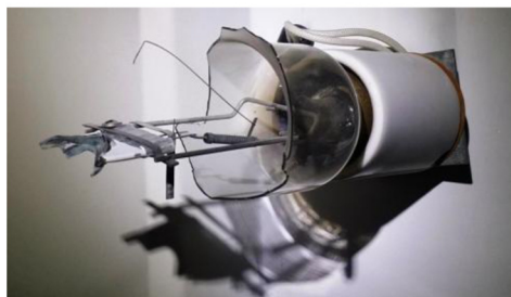
Figure 2. Metal-halide bulb non-passive failure.
