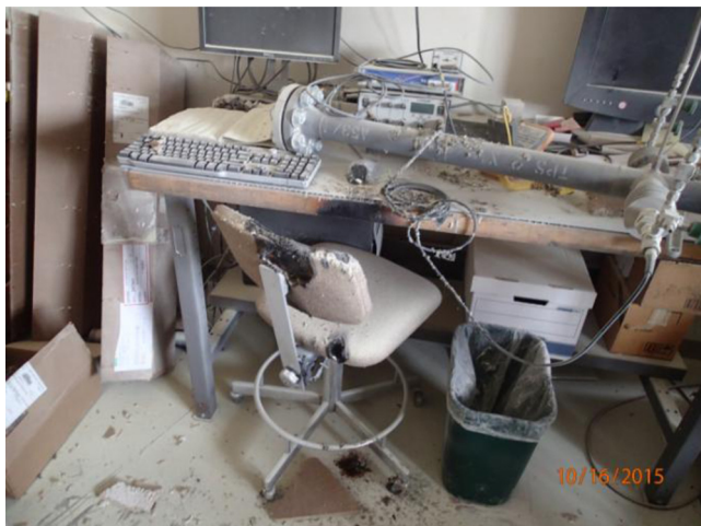
Figure 1. Serious property damage after a metal-halide bulb non-passive failure.
