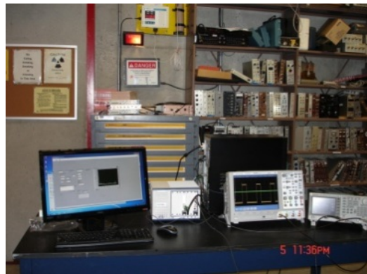
Figure 2.14 The high-speed data acquisition system.
