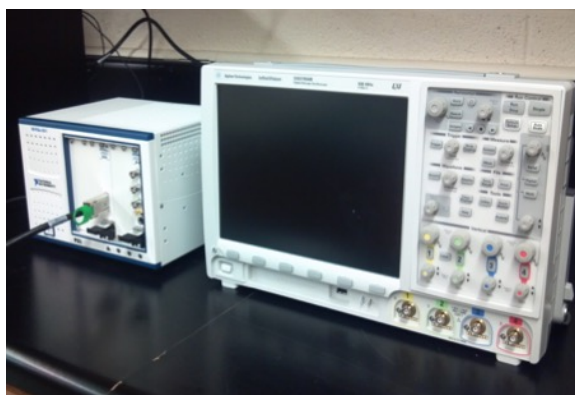
Figure 2.3 High speed digitization system based NI PXIe-5122.
