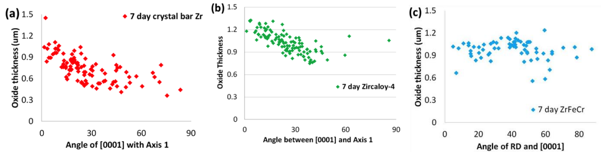
Figure 21: Oxide thickness as a function of grain orientation for crystal bar, Zircaloy-4, and ZrFeCr oxidized for 7 days. Axis 1 represents the normal to the metal surface.
