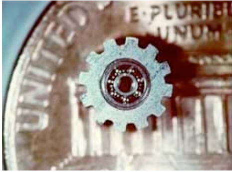
LIGA-micromachined gear for a miniature electromagnetic motor.
