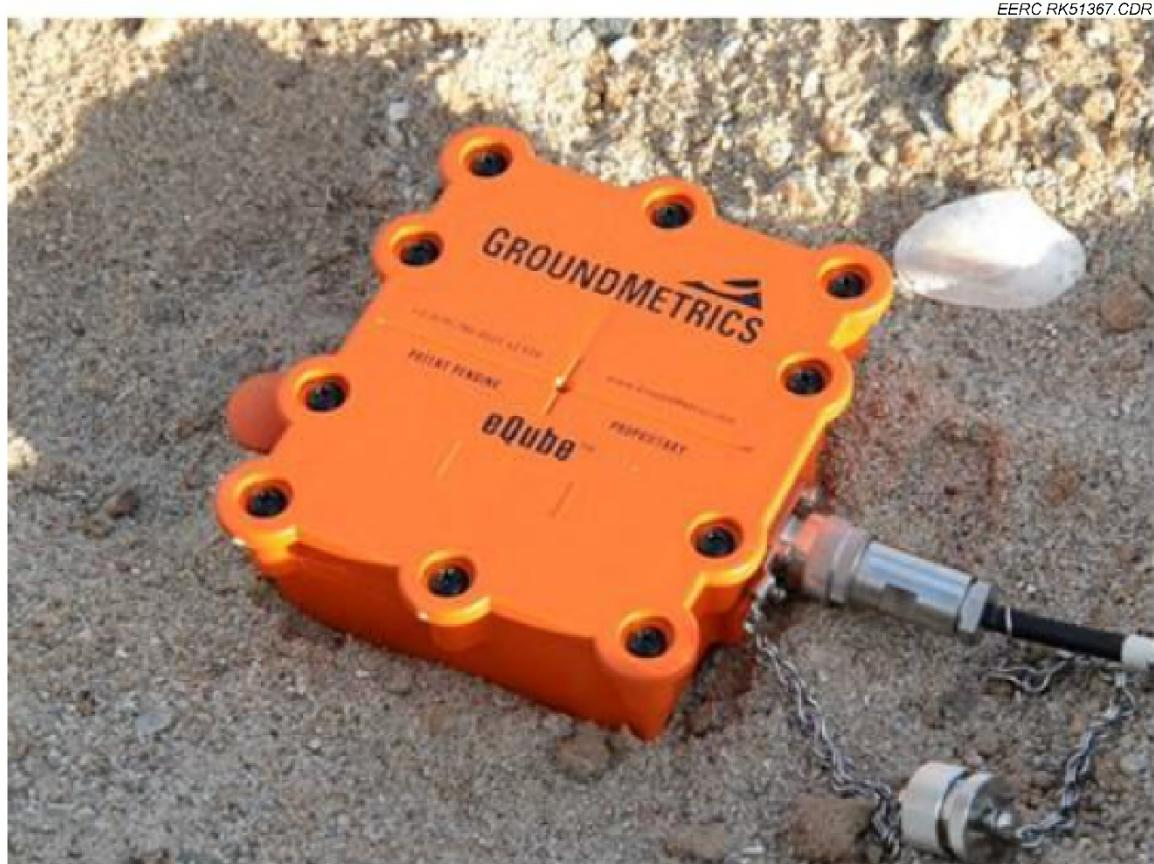
Figure A-42. Surface sensor used in borehole to surface EM surveys. An array of several hundred sensors are deployed on the surface during the survey (courtesy GroundMetrics).
