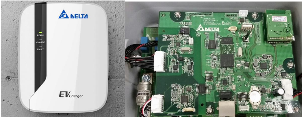
Figure 4: 2 nd -Generation Prototype, verified and shipped to DOE National Labs in October 2014. Left - external view. Right – close-up view of main PCB inside prototype
