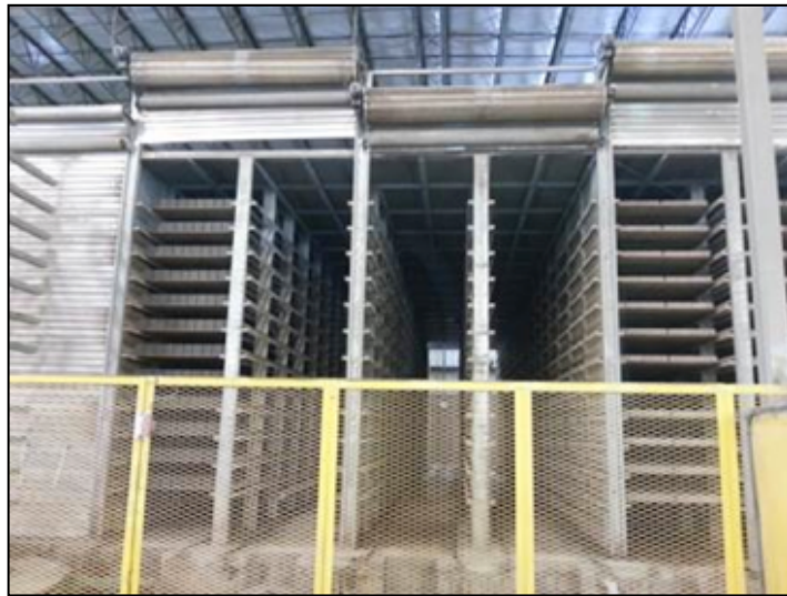
Figure 42. Paver and Block Manufacturer #2's curing chambers with roll-down doors
