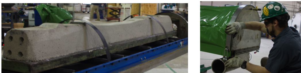
Figure 33. Railroad tie loaded onto curing cart (left) and sealed prior to carbonation (right)
