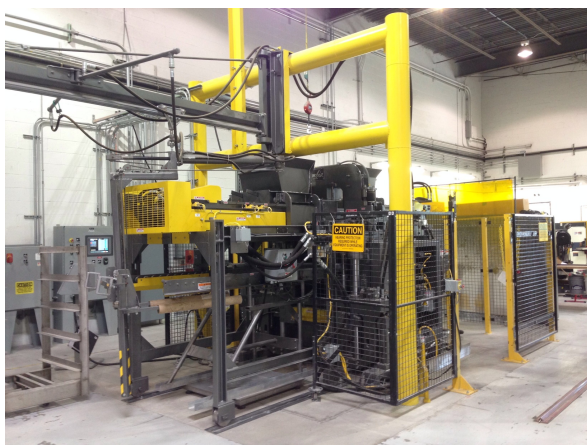
Figure 28. Columbia block and paver press
