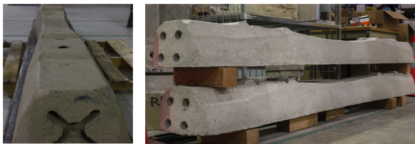
Figure 32. Solidia Concrete railroad tie before (left) and after (right) CO 2 -curing
