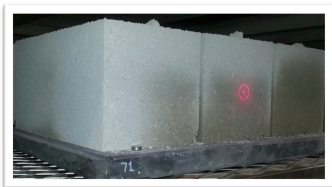
Figure 29. Unevenly dried Solidia Concrete CMUs
